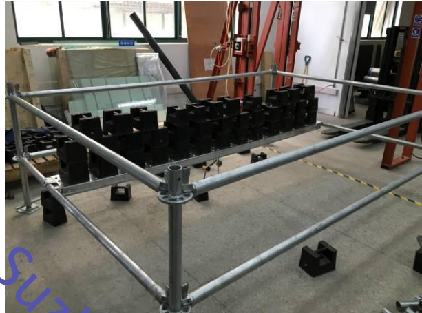
Uniformly distributed load test for 10'
